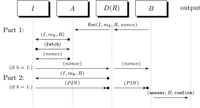
**Fig. 4.** Main phase of  $\pi_{L\text{-Conf}}$  realizing  $\mathcal{F}_{\text{CONF}, \mathcal{D}}(B, I)$  using authenticated and confidential channels drawn as  $\bullet \rightarrow$  and  $\rightarrow \bullet$ , resp. The protocol is between the human initiator  $I$ , his personal device  $A$ , the ATM  $D(R)$  and the bank  $B$ . The bit  $b \in \{0, 1\}$  indicates, whether  $I$  wants to confirm, hence  $(\text{nonce})$  and  $(\text{PIN})$  are only sent in this case.
